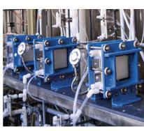
The easy way is to deploy our lab cells. We can feed HCl from your plant directly to 1 dm<sup>2</sup> cells to test the impact on performance. Alternatively, we can spike HCl feeds here.
