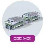
Membrane electrolyzer technology using oxygen-depolarized cathode (ODC): cuts energy consumption by about 30%, reducing the indirect carbon dioxide emissions involved in production.
