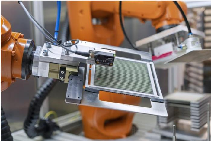
Fully automated assembly of individual components into high-temperature electrolyzers (SOC) and high-temperature fuel cells
